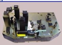
Power workholding fixtures are an effective way to increase productivity, enhance quality, reduce labor and minimize part-to-part changeover times.
